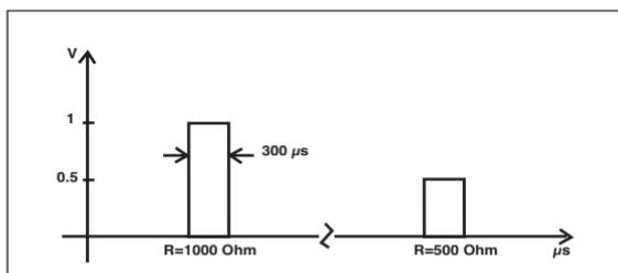
The maximum supplied current is the function of the resistance and of the duration selected, as shown in the following figure:
